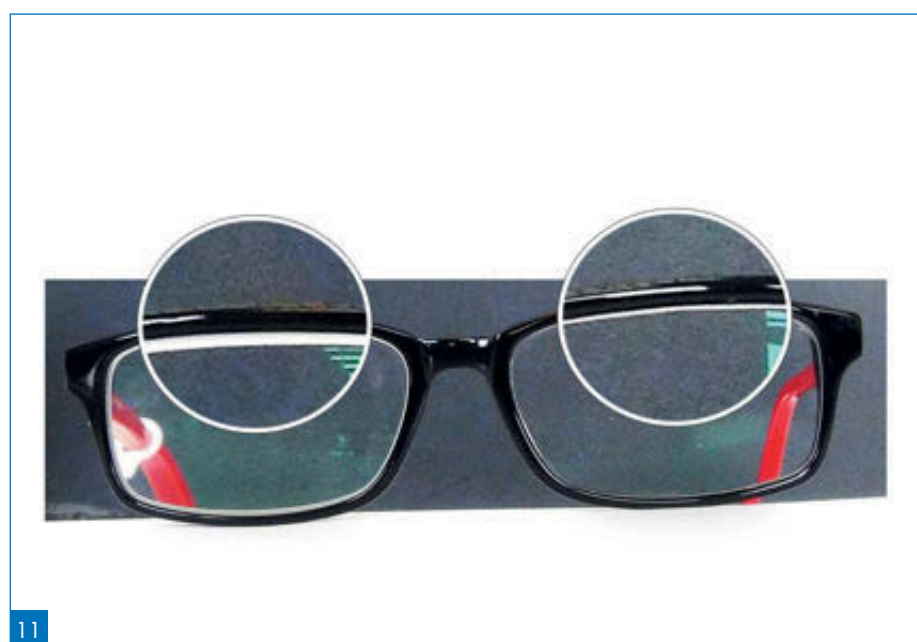
11 Comparison of lenses edged based at conventional tracer data and based at the geometry of the opening in the frame.
